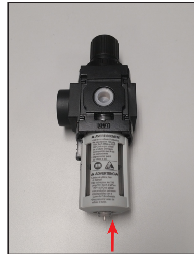
Fig. 1: Draining accumulated water in air filter
