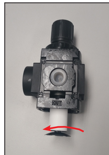
Fig. 3: Replacing air filter
